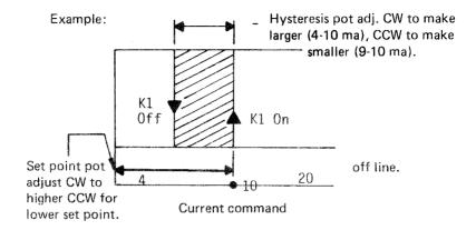
Step 8: (Continued) Set point pot can be set full range (Adjust CW) of input (4 to 20 ma). Example: set point at 10 ma because customer does not want motor to ever be below 10 ma. Relay K1 will stay on as long as input command is above 10 ma. When command goes below 10 ma K1 will shut off (opening K1 contacts).
